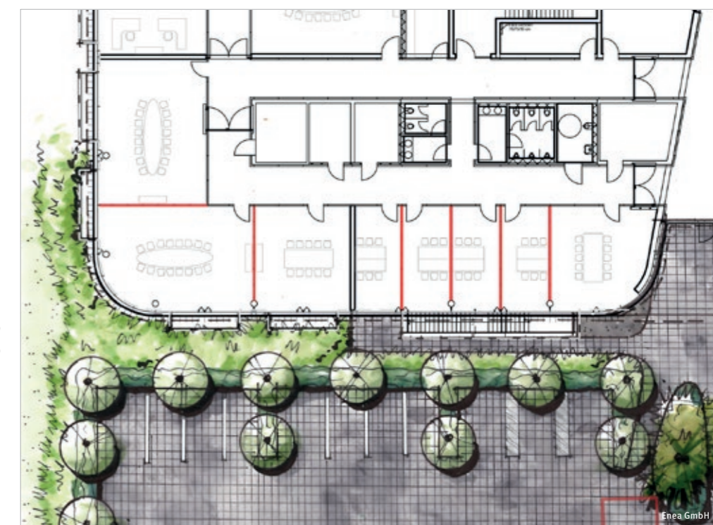
Variable room layout: Flexible walls (marked in red) guarantee a demand-oriented use. The direct connection to outdoor spaces offers high comfort and a pleasant working environment.
