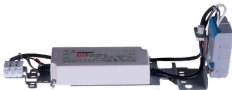
LED operating device carrier (BT) including fixing material (4x spacer bolts(DH) M4x45mm, 2xspacer sleeves (DH) 4mm high, Ø 8mm, for luminaire CAMPO "7700" additional 4 x spacer bolts M4x20mm for extension of spacer bolts M4x45 to 65mm 6x threaded screws (S1) (S2) M4x16mm, 3x tooth lock washer 4.3mm)
